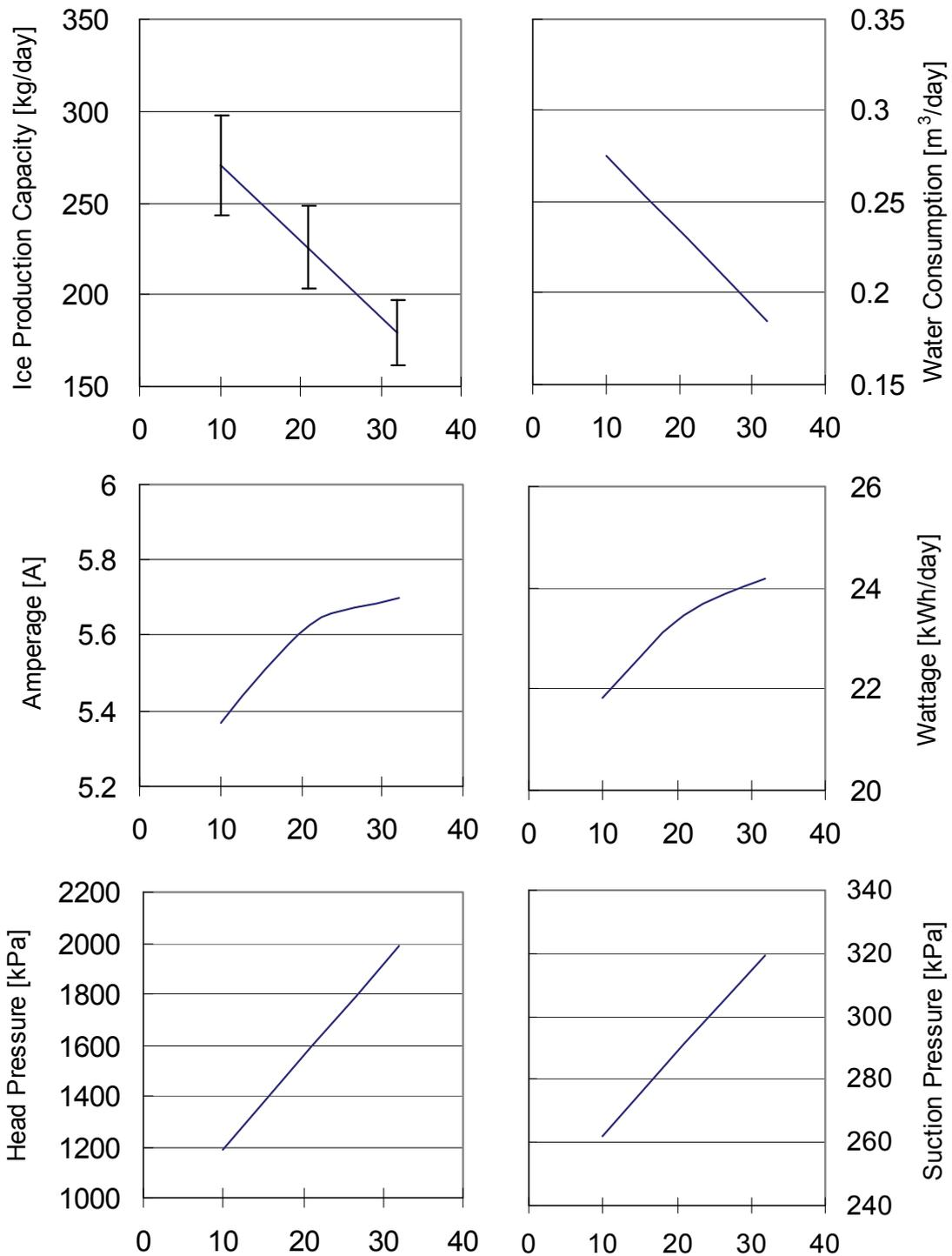
The horizontal axis shows the ambient temperature.
