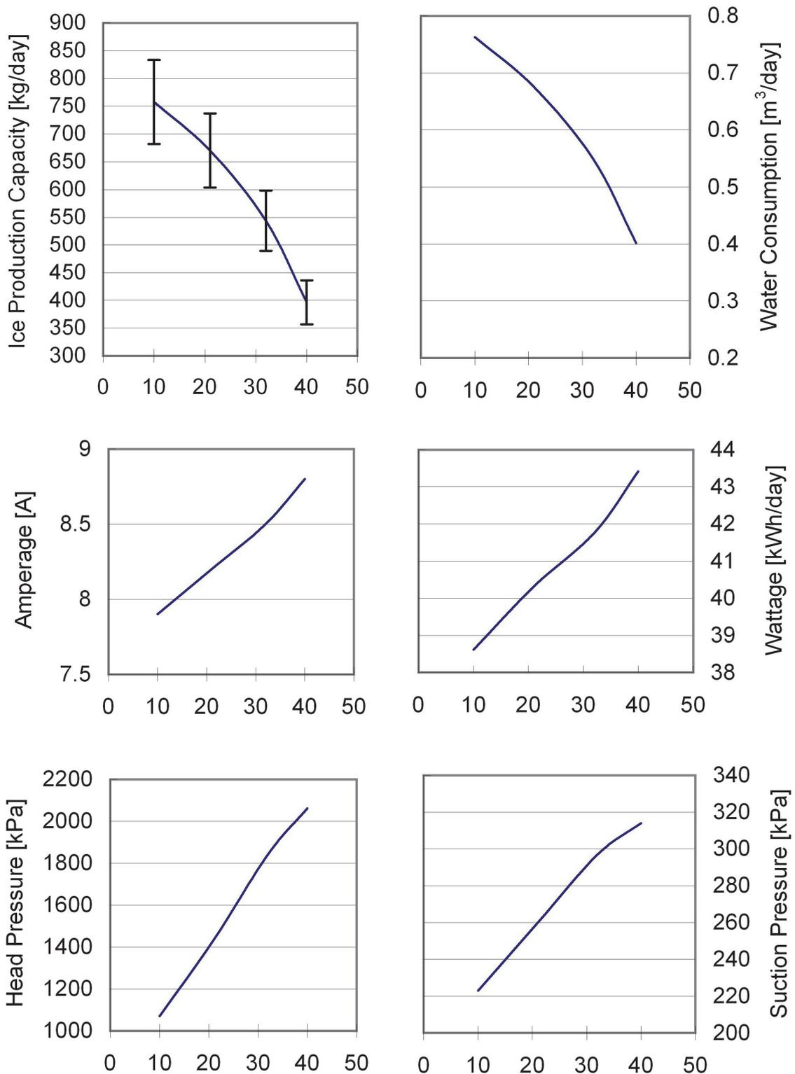
The horizontal axis shows the ambient temperature.
