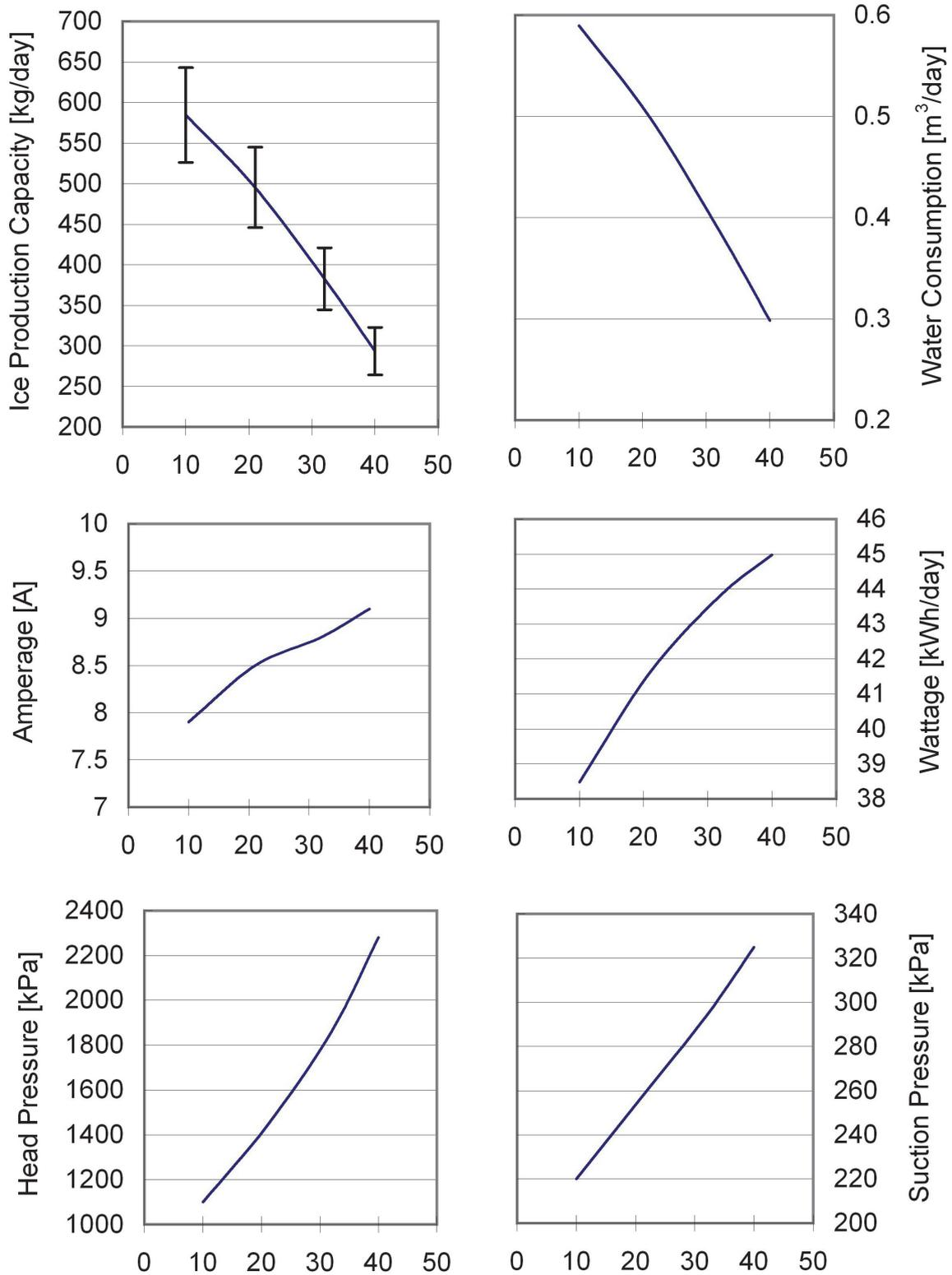
The horizontal axis shows the ambient temperature.
