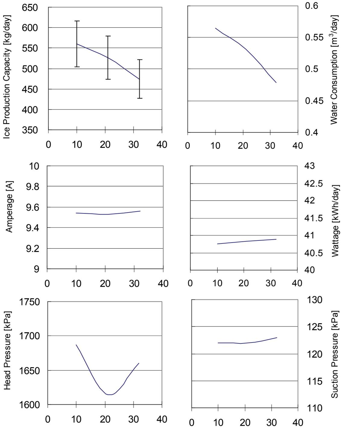
The horizontal axis shows the ambient temperature.
