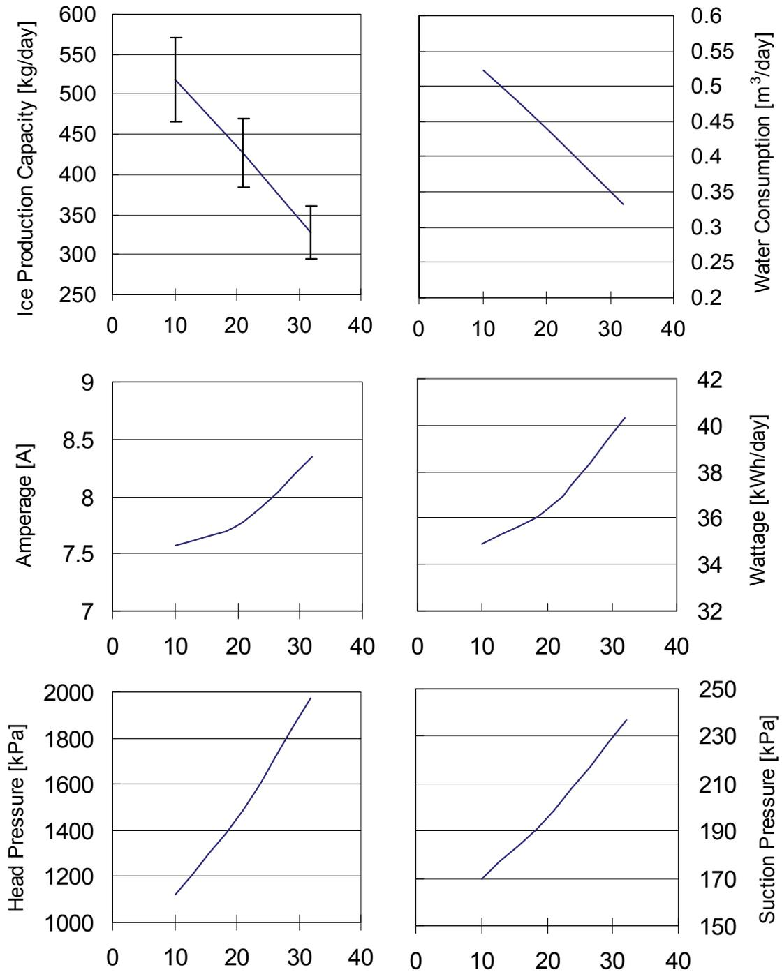
The horizontal axis shows the ambient temperature.
