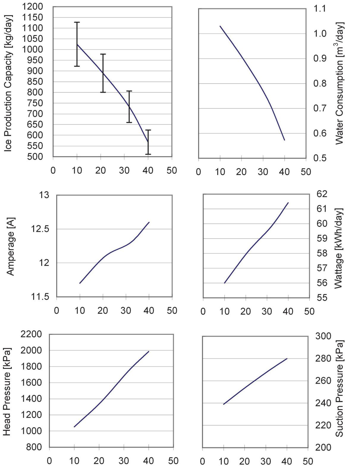
The horizontal axis shows the ambient temperature.
