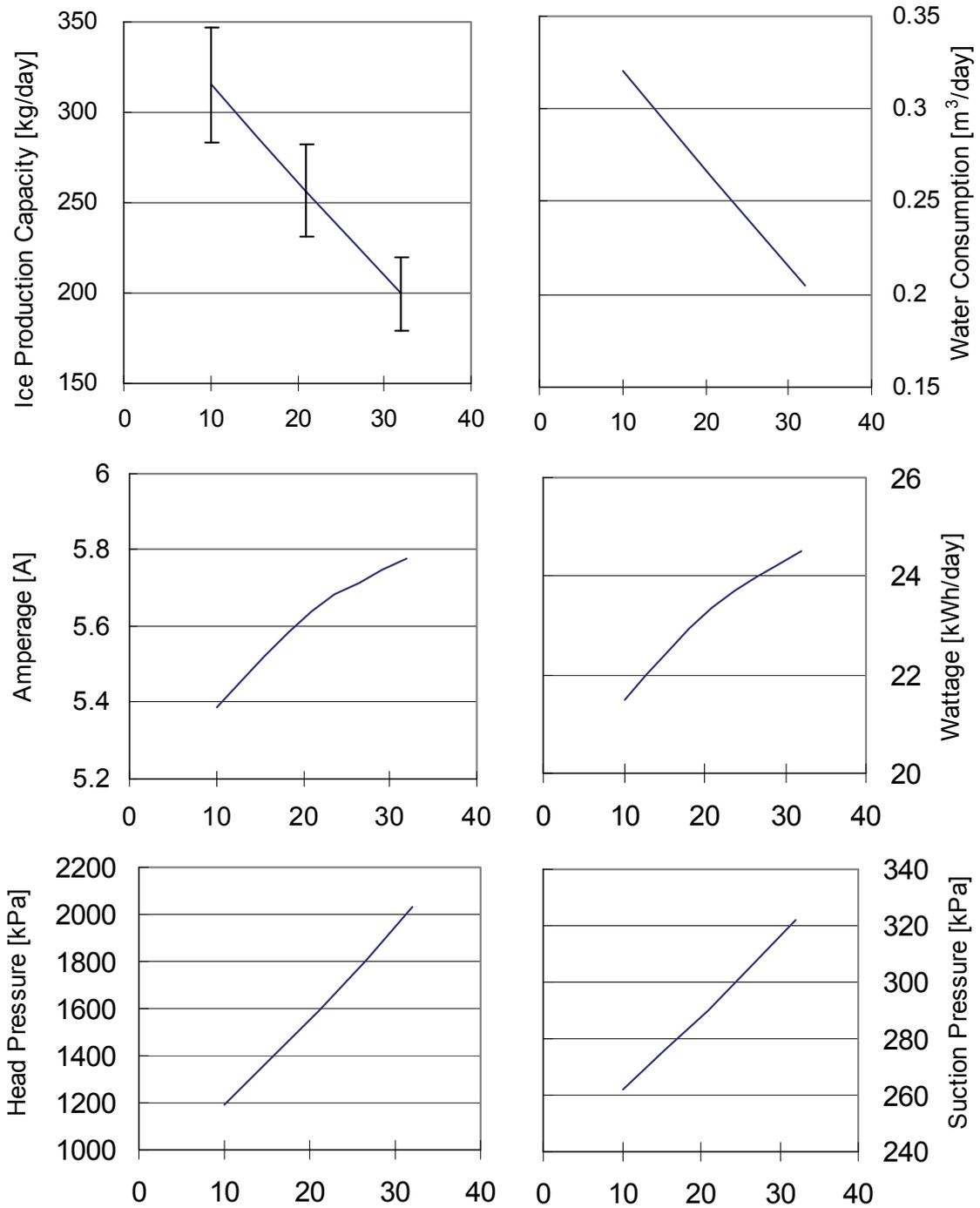
The horizontal axis shows the ambient temperature.
