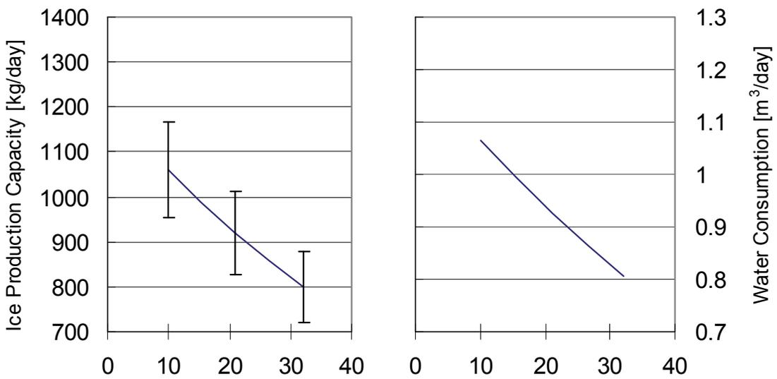
The horizontal axis shows the ambient temperature.
