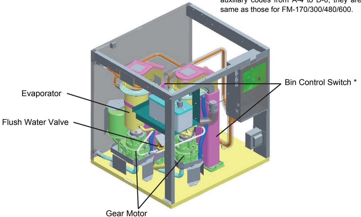
The bin control switch and spout have been changed from D-1. See "[g] BIN CONTROL SWITCH AND SPOUT" for reference.
