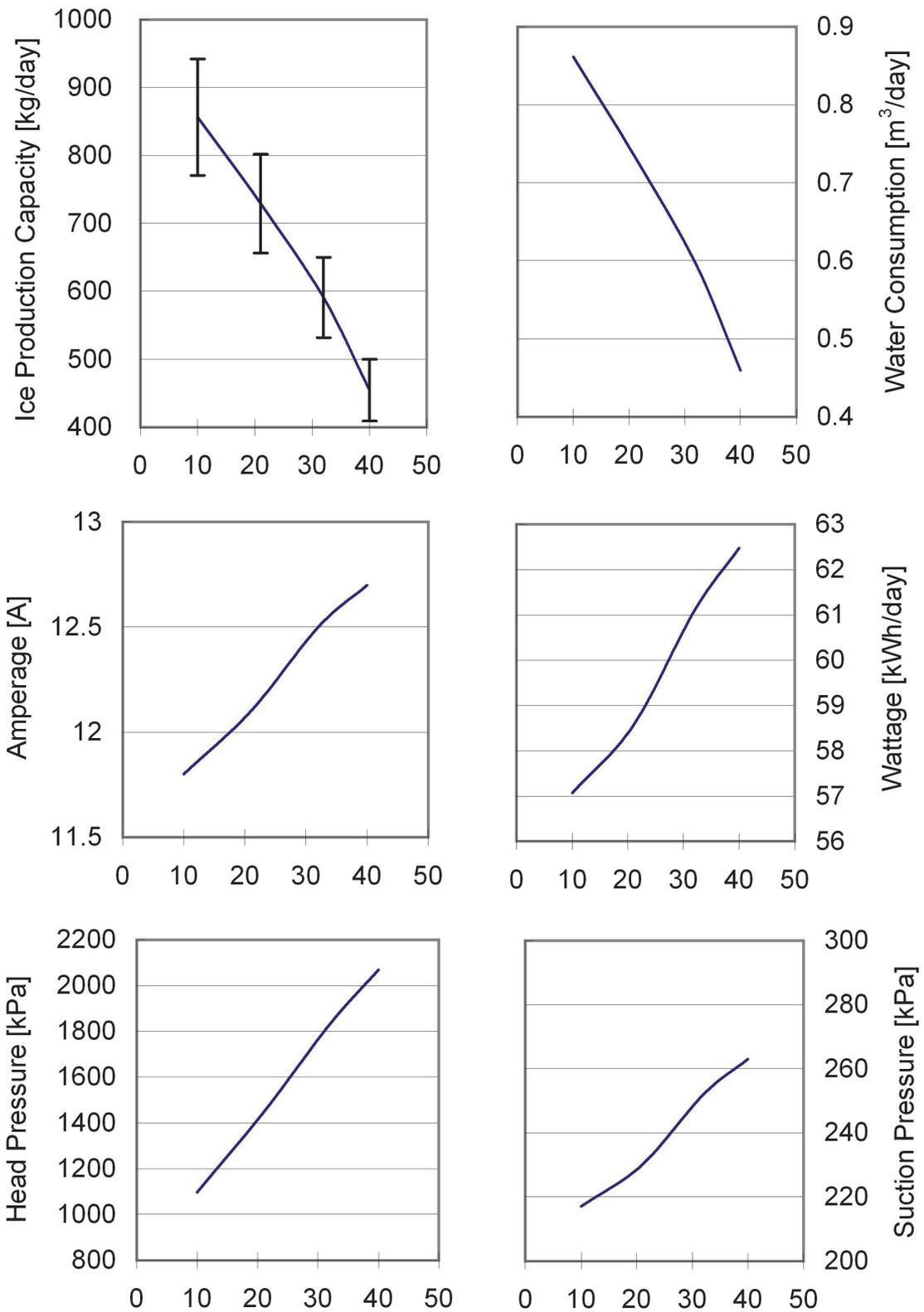
The horizontal axis shows the ambient temperature.
