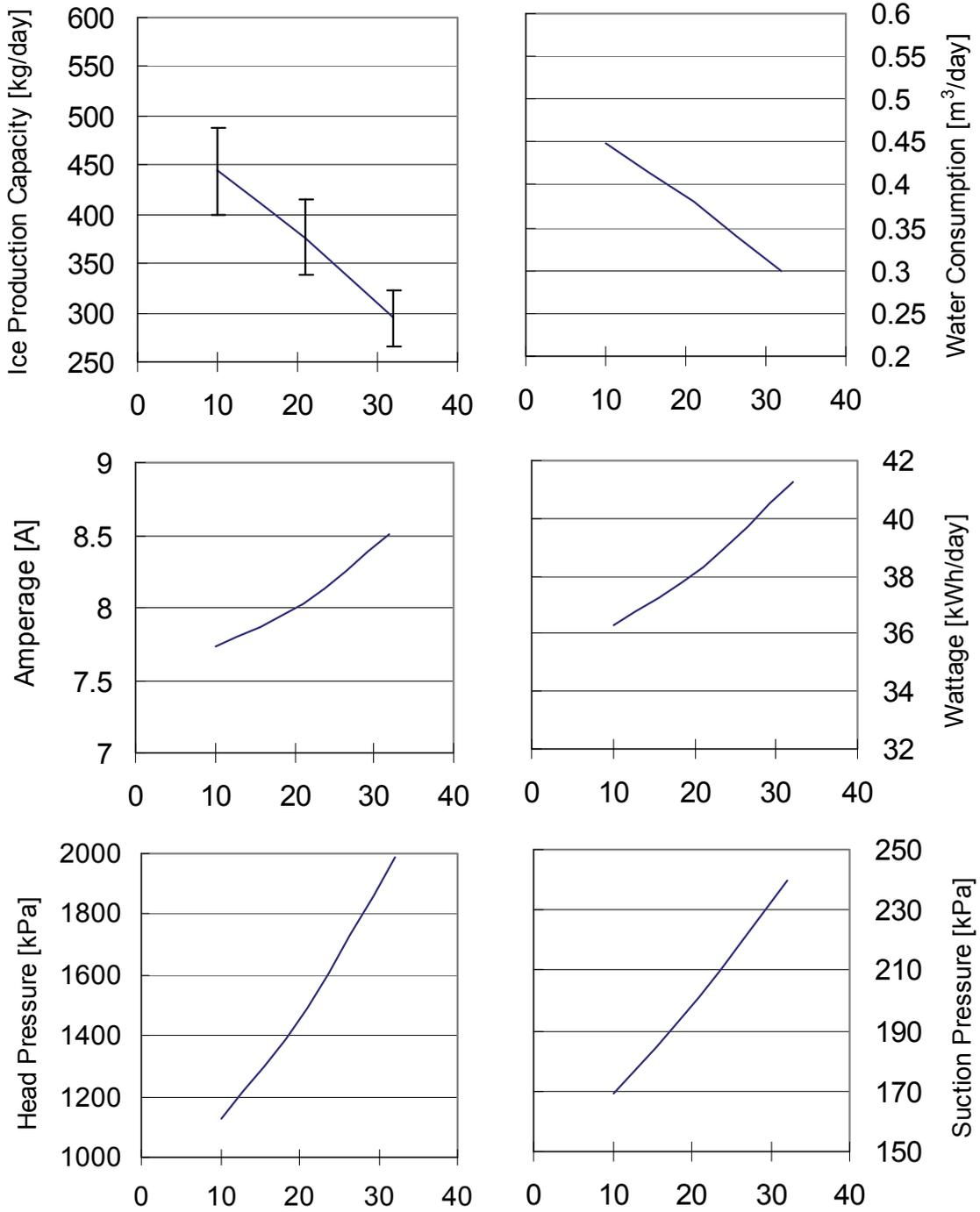
The horizontal axis shows the ambient temperature.
