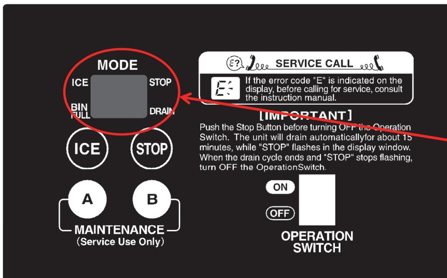
When an error occurs, "E\_" or "c\_" will appear in the display. Some of the "c\_" errors are not displayed and must be checked by the error log.
