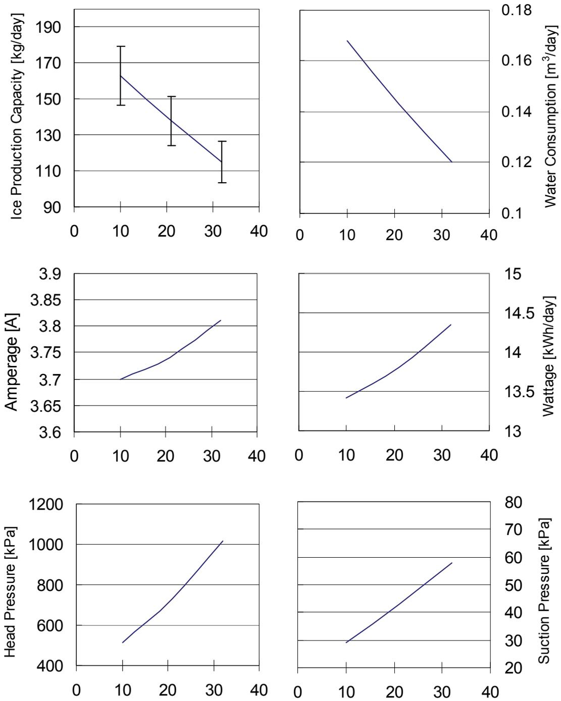
The horizontal axis shows the ambient temperature.
