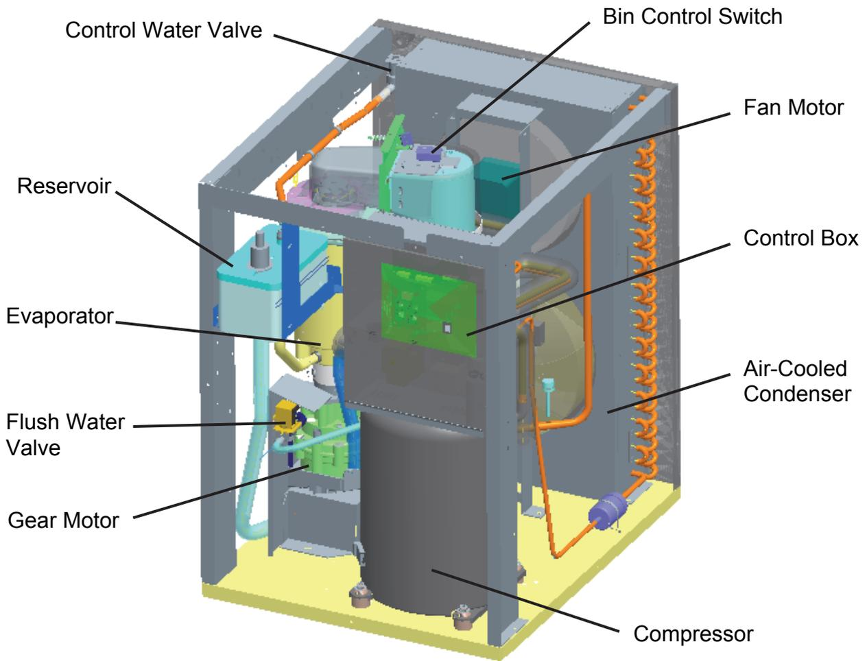
The bin control switch and spout have been changed from D-1. See "[g] BIN CONTROL SWITCH AND SPOUT" for reference.
