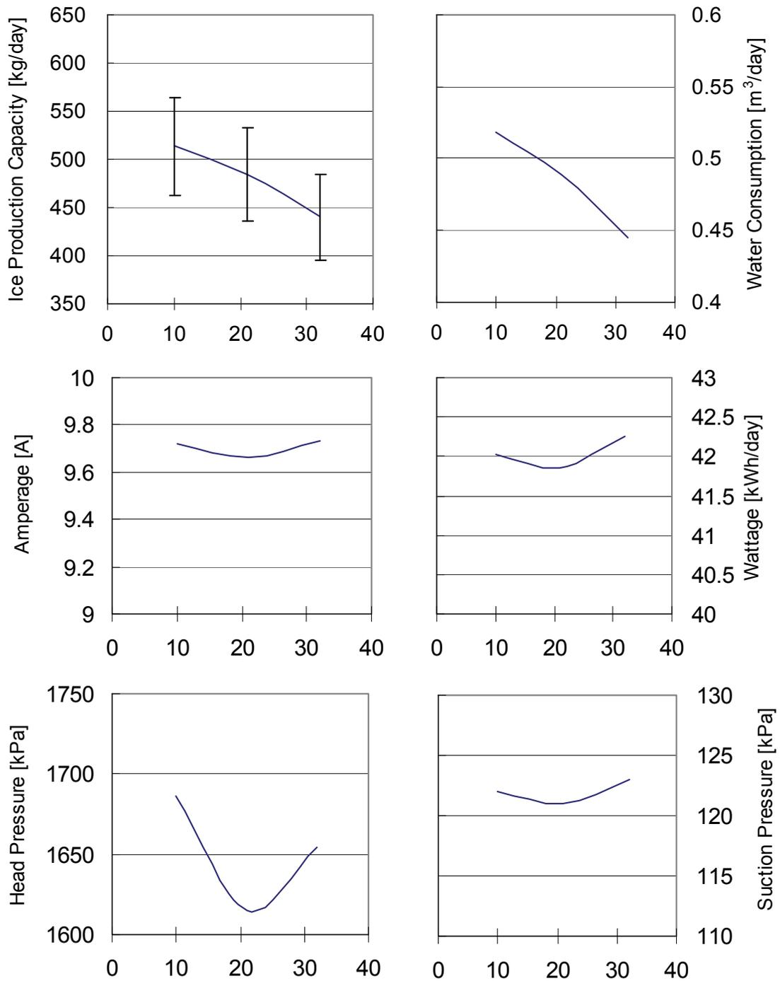
The horizontal axis shows the ambient temperature.
