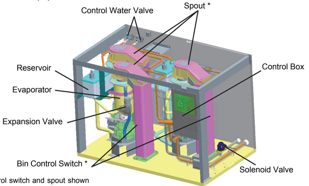
\* The bin control switch and spout shown here are for the auxiliary code A-3 or earlier. For the auxiliary codes from A-4 to D-0, they are the same as those for FM-170/300/480/600.
