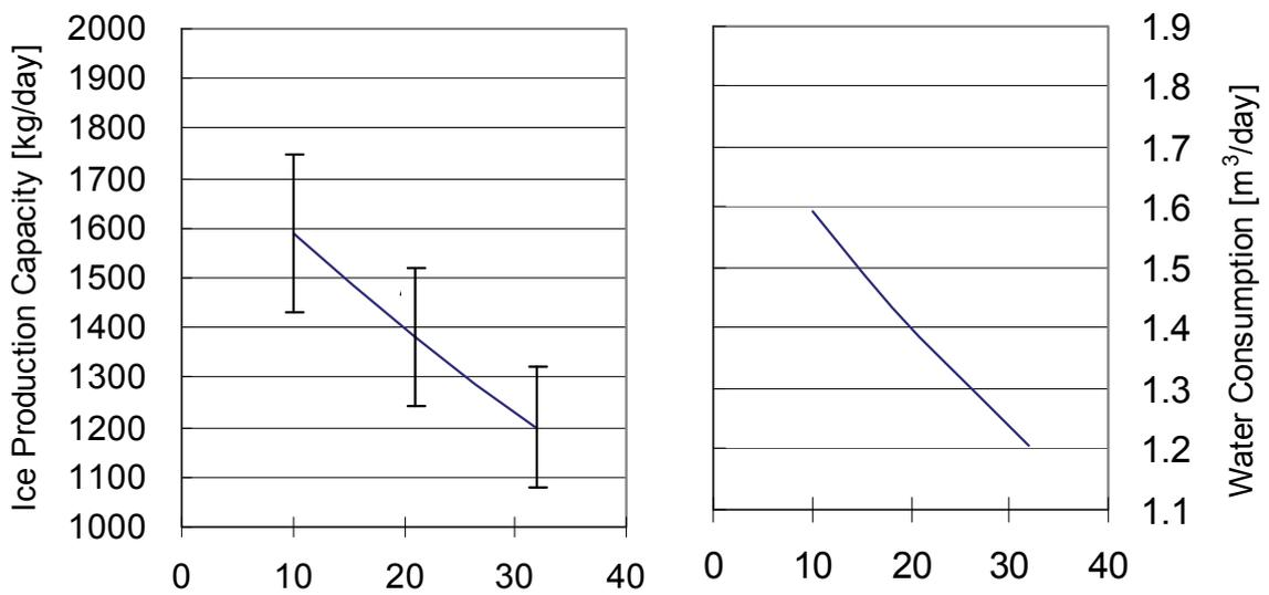
The horizontal axis shows the ambient temperature.
