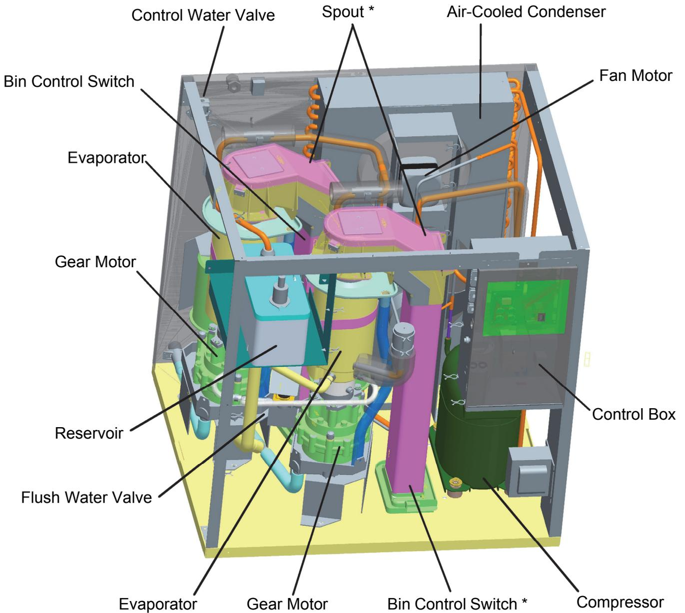
\* The bin control switch and spout shown here are for the auxiliary code A-2 or earlier. For the auxiliary codes from A-3 to D-0, they are the same as those for FM-170/300/480/600.
