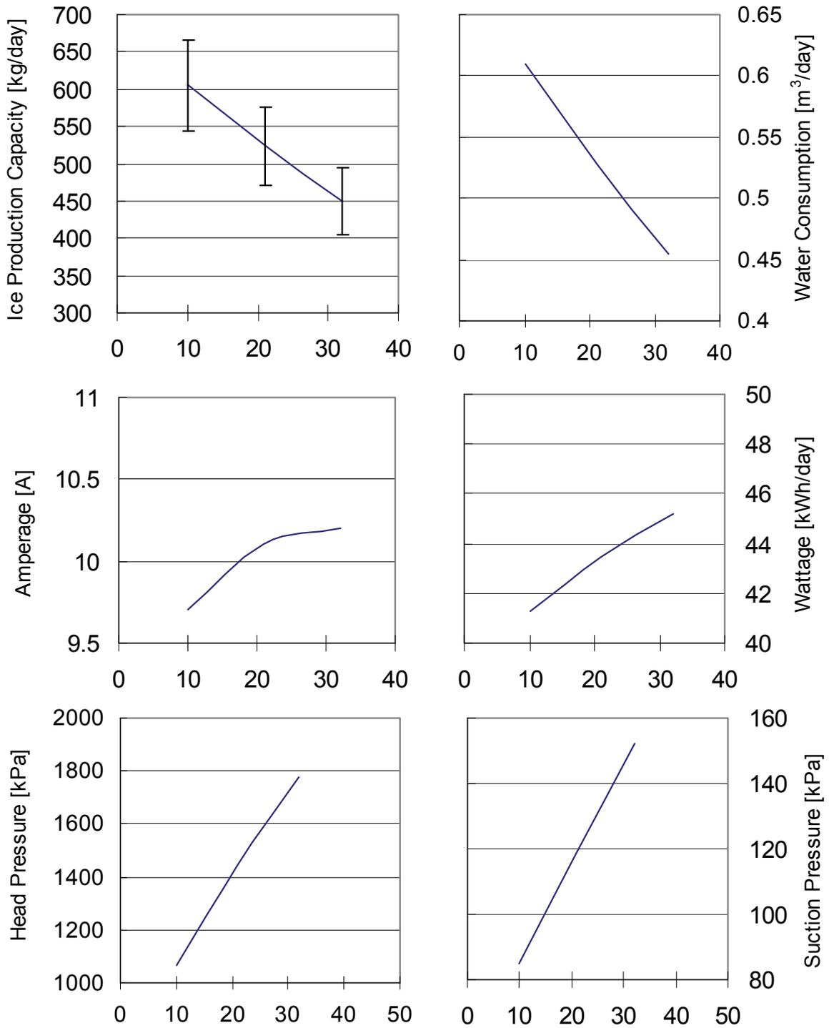
The horizontal axis shows the ambient temperature.
