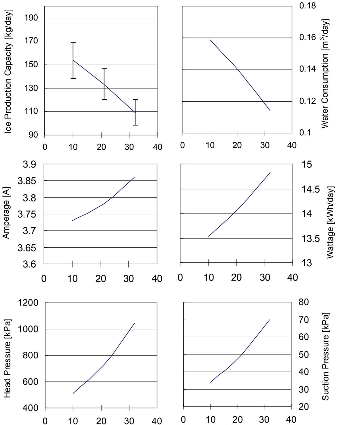
The horizontal axis shows the ambient temperature.
