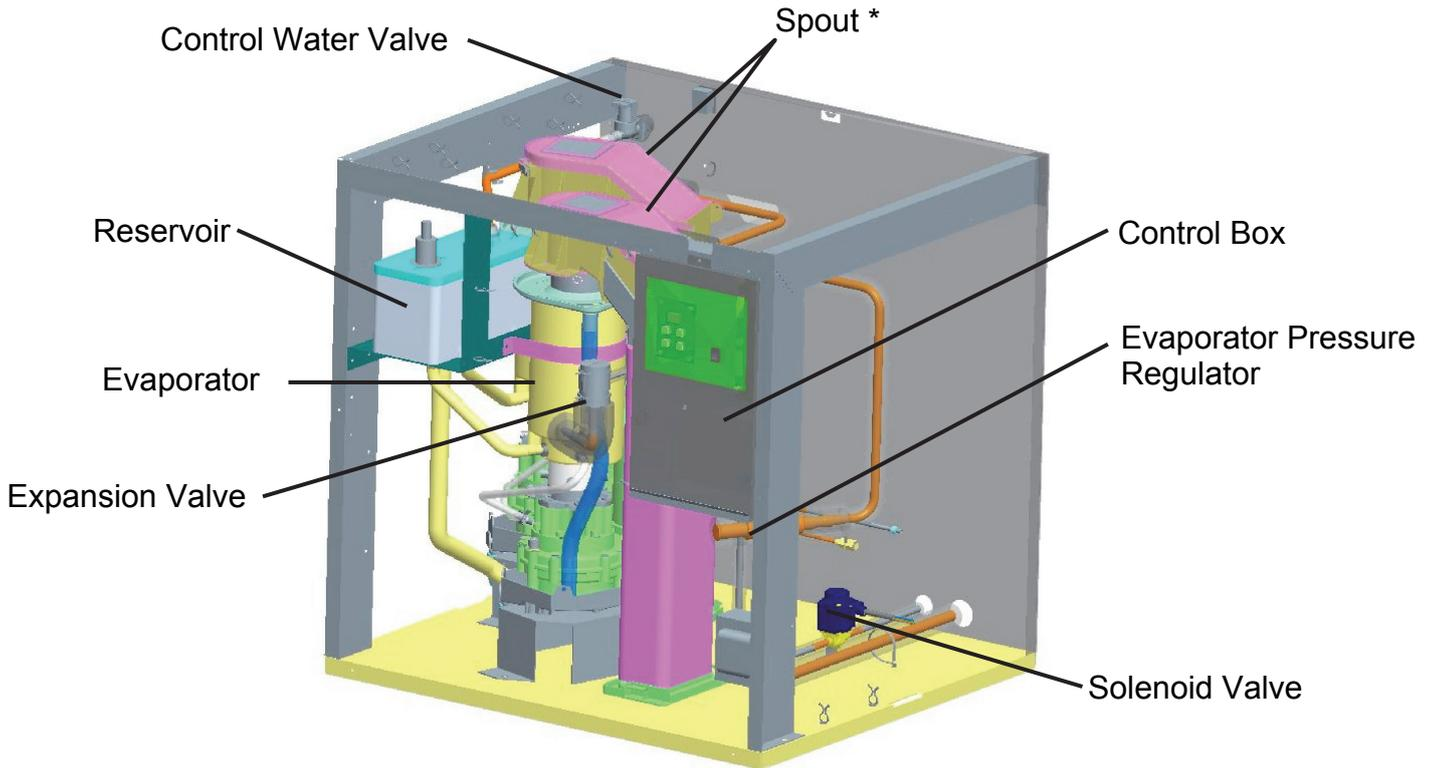
\* The bin control switch and spout shown here are for the auxiliary code A-3 or earlier. For the auxiliary codes from A-4 to D-0, they are the same as those for FM-170/300/480/600.
