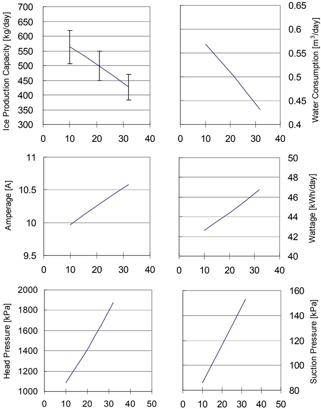
The horizontal axis shows the ambient temperature.
